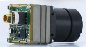
**DA:** **The world's smallest and lightest VGA format thermal imager** for thermal imaging applications that require minimum volume and weight. Enables new applications in smaller packages. Offers low power consumption, high shock and vibration tolerance, and affordability. **Size (w/o lens): 17 x 22 x 22 mm; Weight (body & lens): 23 g (13mm lens) <-> 28g (35mm lens)**
