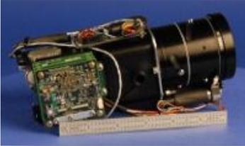
**Product:** Eagle MWIR 640A, 40x480 pixel format SWIR integral Stirling cooled, high performance camera system. The camera system development was derived from the 640x512 SWIR electronics developed by Nova and took only three months from concept to camera operation
