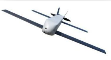
**DA:** Miniature UAV with ISR and strike capabilities that can be quickly launched from diverse battlespace conditions.
